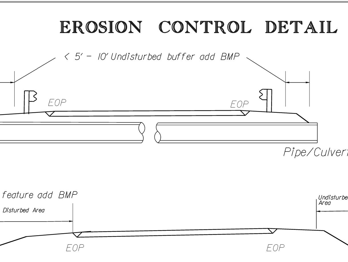
Use BMP's if berms, shoulders and/or frontslopes and/or ditchline and/or backslopes are disturbed
